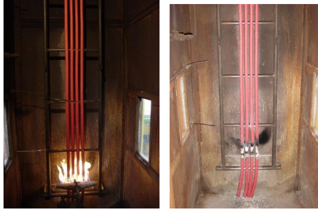
Figure 11 : EN 50399 apparatus (courtesy from Nexans)
