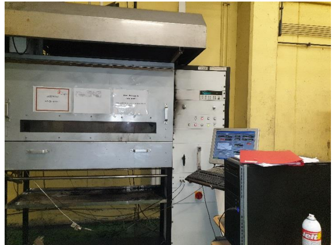
Figure 2 : EN ISO 9239-2 Flooring radiant panel test [30].
