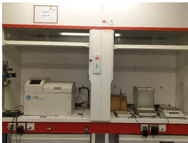
Figure 7 : ISO 1716 apparatus (courtesy form CREPIM)
